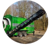
Extended conveyor belt for middle fraction
