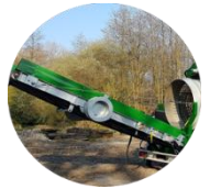
Extended conveyor for coarse fraction
