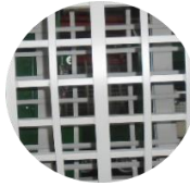
Bisection of the inner trommel approx. 75 x 75 mm
