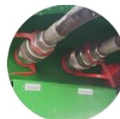
Additional connector for powering an additional conveyor
